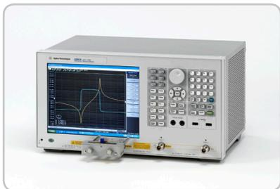
Gain-phase series-thru method using 16047E 4TP fixture
